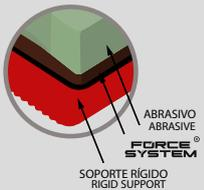
The construction of the tool combining flexible with rigid parts guarantees a perfect coupling and a constant contact on surfaces, **avoiding marks and scratches on the polish**. We recommend applying **Force System technology on the finest grains** to achieve the highest polishing and shining quality.
